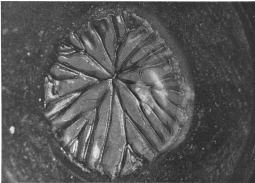
FIG. 7. The corrosion relief of NaCl, c_0 = c_{\infty} = 0.010 \text{ g/cm}^3 , mgt. 5
